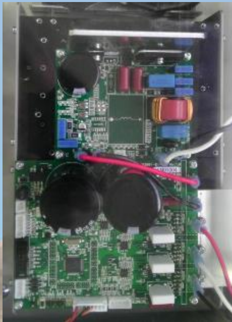
AC/DC/AC Power Converter
