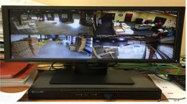
This recorder connect and communicate via HDMI port, lan port. Once the manually set Ip for each cameras connect to recorder. Recorder processor support 10/1000 Base T Ethernet which have high speed communication using TCP/IP.
